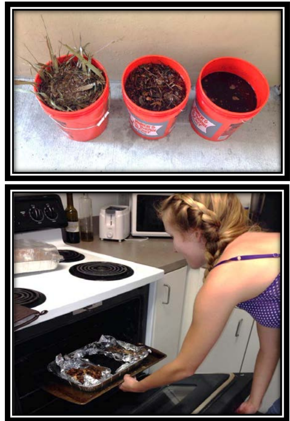
Figure 3: Above- Substrates were submerged in water in order to reach 100% moisture content. Below- To reach 55-65% moisture percentage, substrates with excess moisture were baked at 350°F for 15 min intervals.
